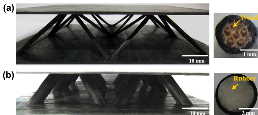
Fig. 3. (a) Wood-core truss (b) silicone rubber-core truss and their corresponding carbon fiber composite pyramidal lattice structures.
